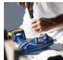
1. Remove the cover with a screw driver.
