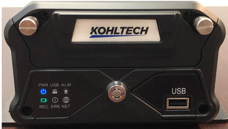
Normal operation - Blue PWR and Green REC
