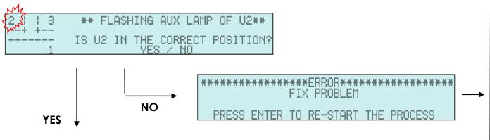
If YES is pressed, the AUX lamp will begin flashing *only* on U3 and the '3' digit in the simulated intersection on the screen will begin flashing:
