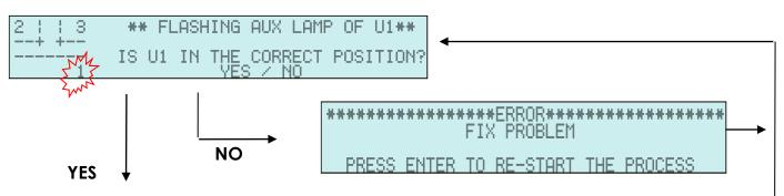
If YES is pressed, the AUX lamp will begin flashing *only* on U2 and the '2' digit in the simulated intersection on the screen will begin flashing:
