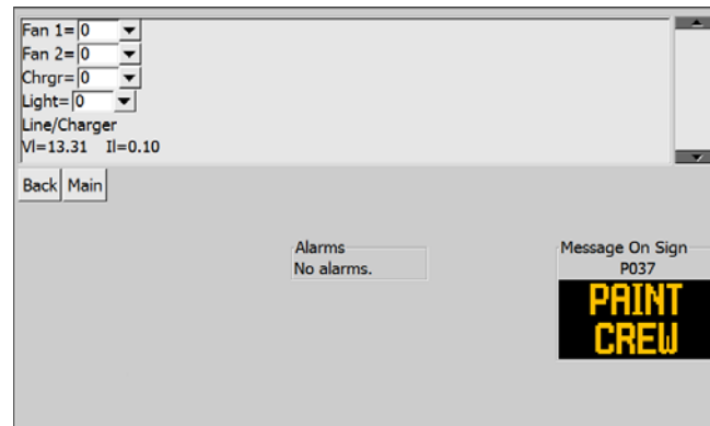
Figure 4-71. Fan & Charger Power screen
