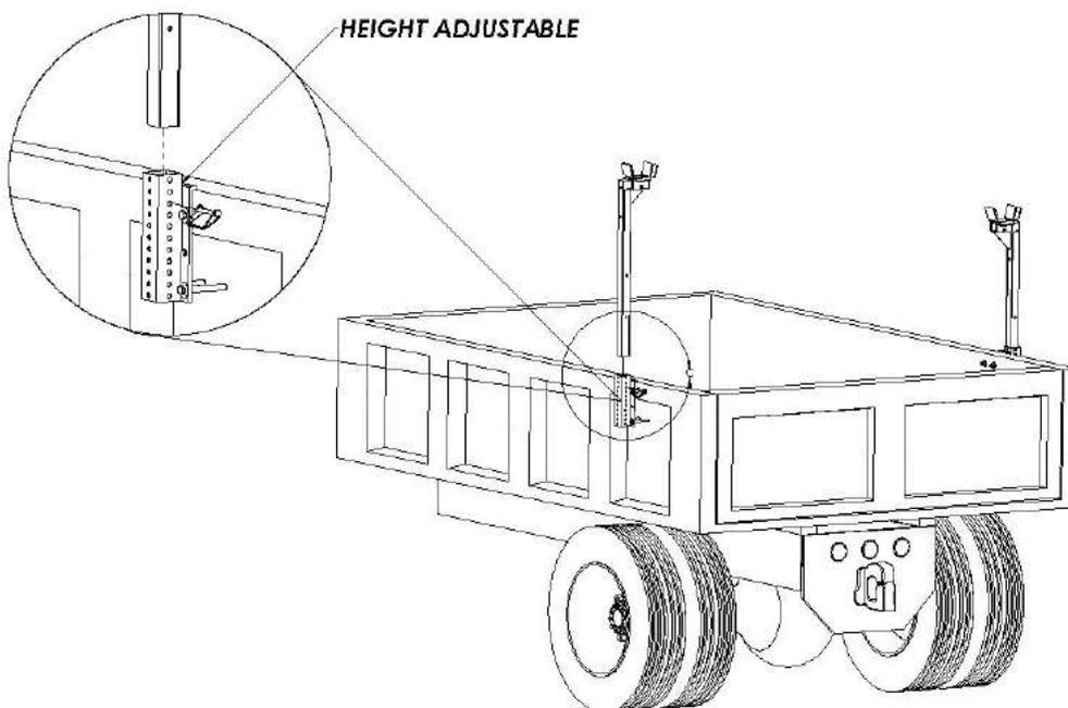
3. To mount the support brace (11057L/11057R), position the brace to where the inside surfaces of the brace face inwards to the truck. Align the hole on one end of the support brace with the hole on the support post. Insert a 1/2" bolt to fasten one side of the support brace, as shown in following figure:
