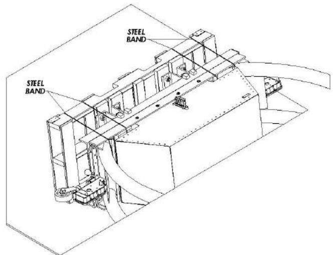
6. Use the forklift to lift the backup end of the cartridge to a sufficient height to deploy the swivel jacks located on the backup as shown in following figure. Crank the swivel jacks and rotate the wheels to the deployed position.
