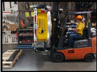
2. Lift the Strut off the pallet using a forklift.
