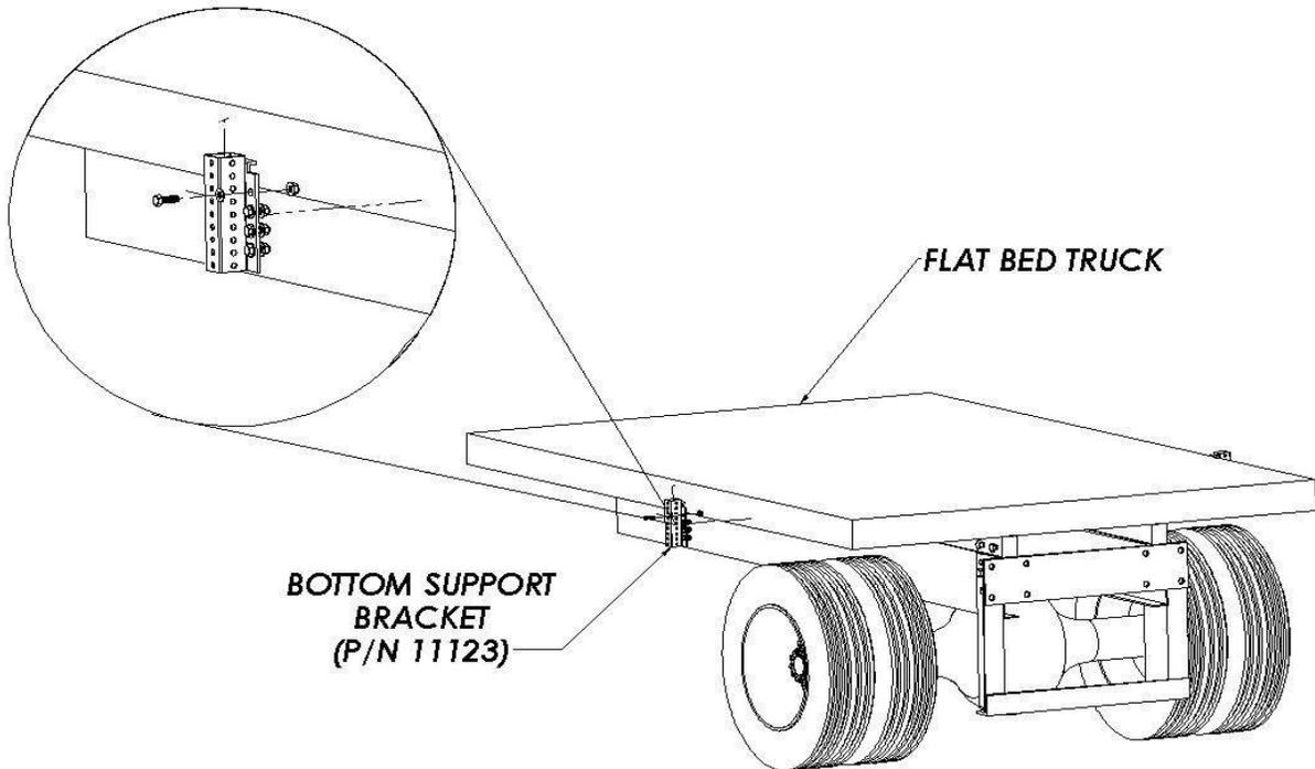
2. Insert the support post into the bottom support bracket. Adjust the post to the appropriate height, which will vary based on the host vehicle, to where the Cartridge tubes will be able to rest on the support post top saddle when the TMA is in the stored position. This figure below illustrates how the support posts can be adjusted upon installation.
