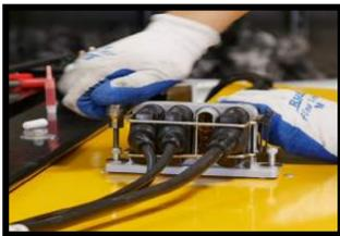
7. Secure junction box, clamp, and connecting power cable.
