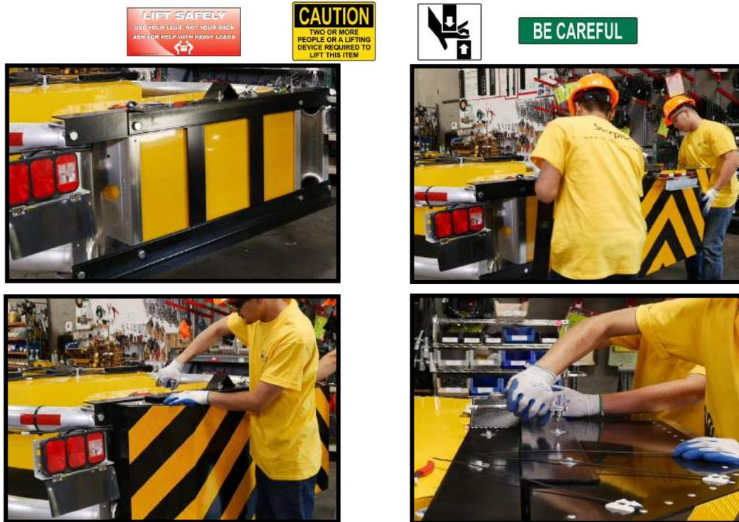
9. Cut the zip tie that is holding the electrical cable and attach it to the cable that is located in the back of Module A. Secure the cables to the top of Module A using zip ties.
