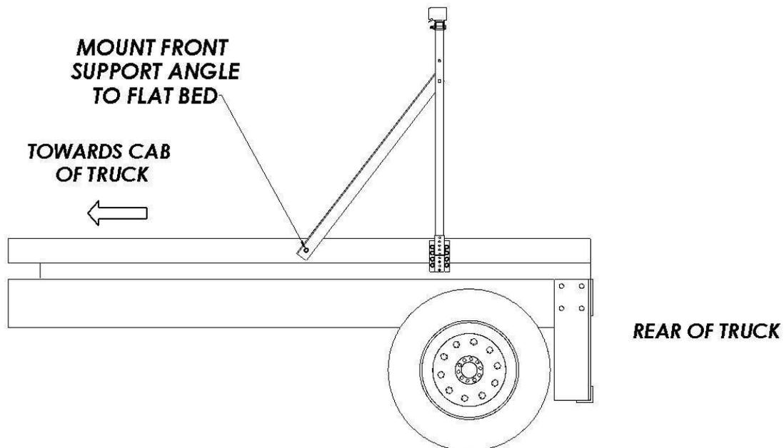
5. Mount the rear support angle to the side support post, with the inside faces of the angle facing outward in the same direction as the front support angle. Pivot the rear support angle towards the rear of the truck, and mark the hole to drill and mount the rear support angle to the bed of the truck. The figure below specifies each location to mount the rear support angle.
