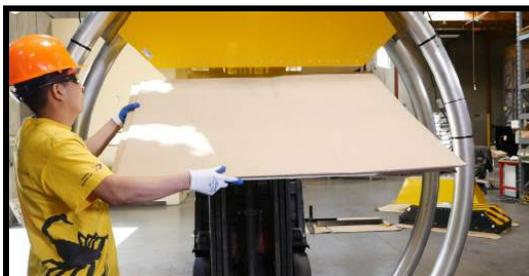
6. Place a piece of cardboard on the forklift to prevent damage to Module B.
