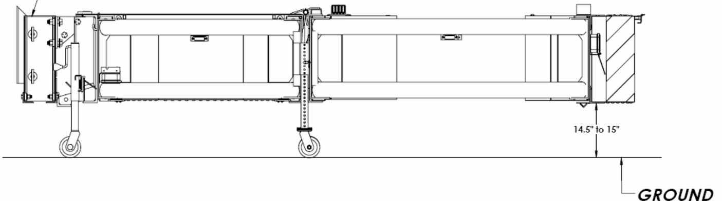
4. Once the TMA is rolled towards the back of the host vehicle, tack weld the tubes in place at the outermost and innermost four corners where the tubes touch the frame. This image below illustrates ideal tack welding locations to hold the tubes in place.
