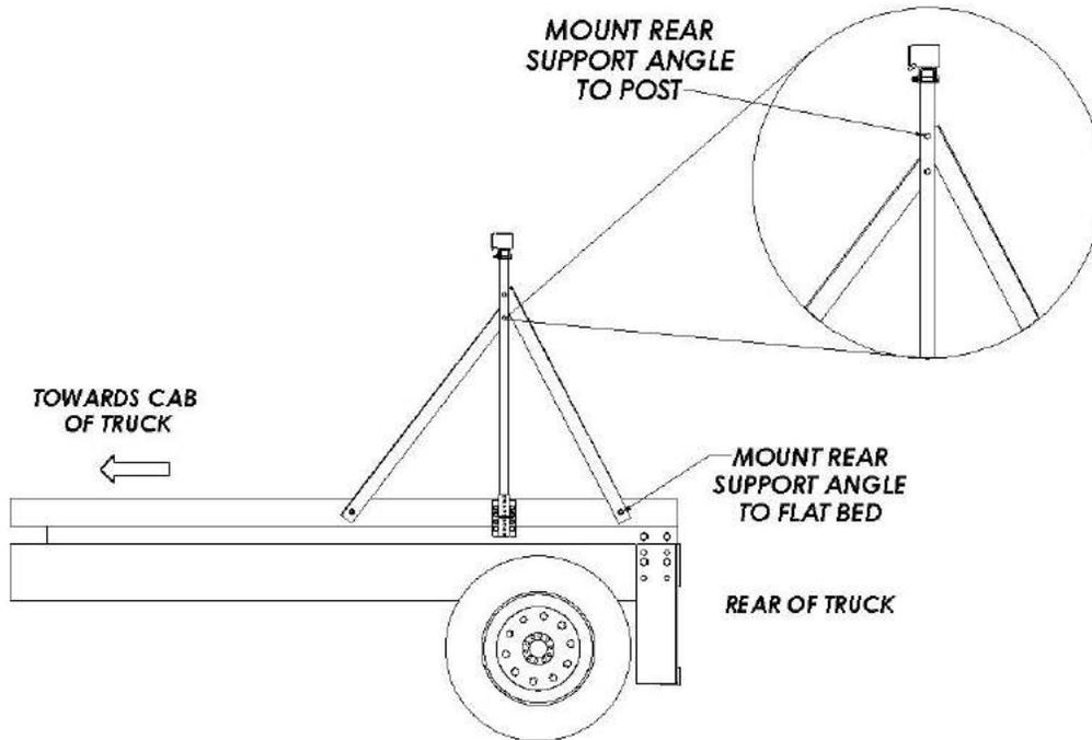
6. When the TMA is raised to the stored position, the wear plates that are mounted onto the top half of the Cartridge tubes (already mounted onto TMA) should align and rest upon the top support post saddles (P/N 11040C) as shown in the figure below.
