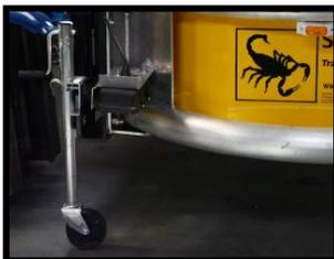
7. Lower the swivel jacks so the Strut is no longer supported by the forklift.
