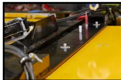
7. Secure the junction box and bolt the clamp on top of Module C. Once secure, connect the power cable to the junction box.
