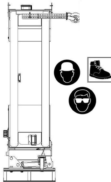
5. Use the forklift to lower the pallet to the horizontal position as shown in the figures below. Verify that the pallet is tipped in the correct orientation with the junction box on top, which can also be seen in the following figure. **Caution – Keep personnel away from the TMA when the steel bands are cut.** Keep clear from pallet when pallet is pulled free of the cartridge for it will drop a few inches. Steel band locations are identified in the figures below.
