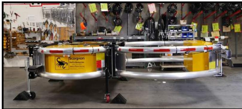
6. Secure the hydraulic cylinders to the Cartridge frame using the clevis pins. Secure the clevis pins with hair pins.
