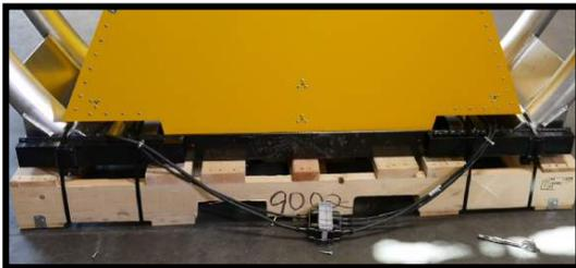
3. Unbolt the junction box from Module C.
