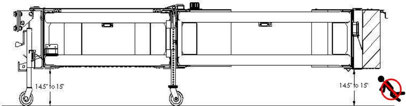
4. With the jacks deployed, roll the deployed TMA to the rear of the host vehicle and align the TMA centerline with the vehicle, as shown in the following figure. The backing plate that is bolted onto the TMA (See step 2) should be flush with the ends of the truck frame.
