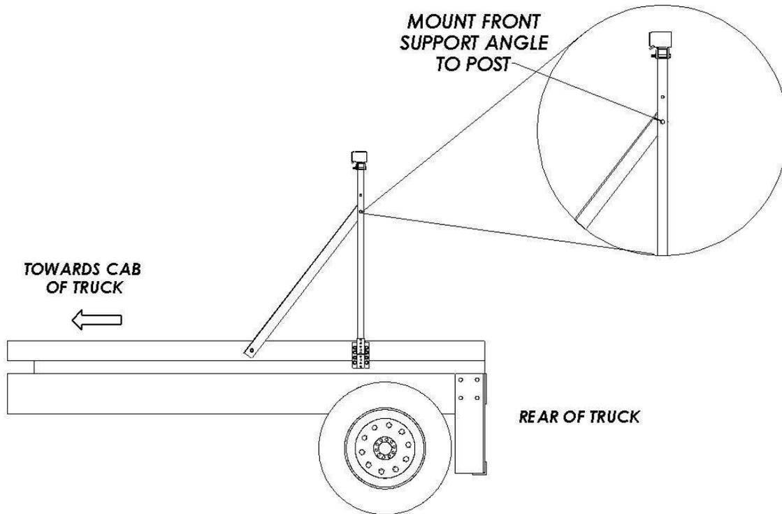
4. Pivot the front angle towards the cab of the truck. Mark and drill another hole into the flat bed and securely fasten the front support angle in place, as shown in the following figure.
