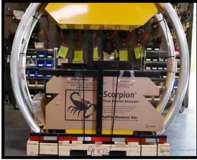
1. Cut and remove Steel bands and cardboard from the Cartridge.
