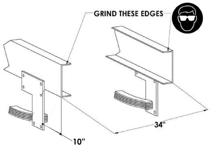
2. Mount the Backing Plate (P/N: 10353) onto the backup of the TMA as shown in this figure (right). Mounting the backing plate onto the TMA will simplify the alignment process when mounting the backing plate onto the truck frame of the host vehicle.
