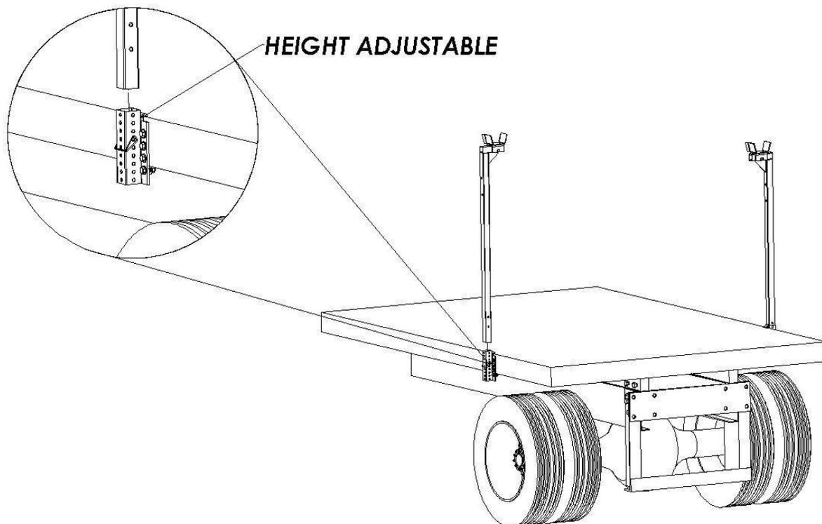
3. To mount the front support angle, position the angle to where the inside surfaces of the angle face away from the flat bed. Align the hole on one end of the front support angle with the hole on the support post, which is the second hole down from the top of the post. Insert a 1/2" bolt to fasten one side of the front support angle, as shown in this image.
