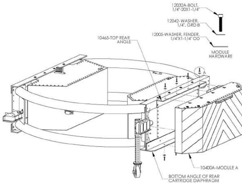
8. The rear ICC bar light (on top of Module A) has two wires extending from it with plugs. Connect the plugs into the electrical wire plugs at the side of the light. Once connected, strap the wire portion of the ICC harness on top of the Module A as shown in the next figure.
