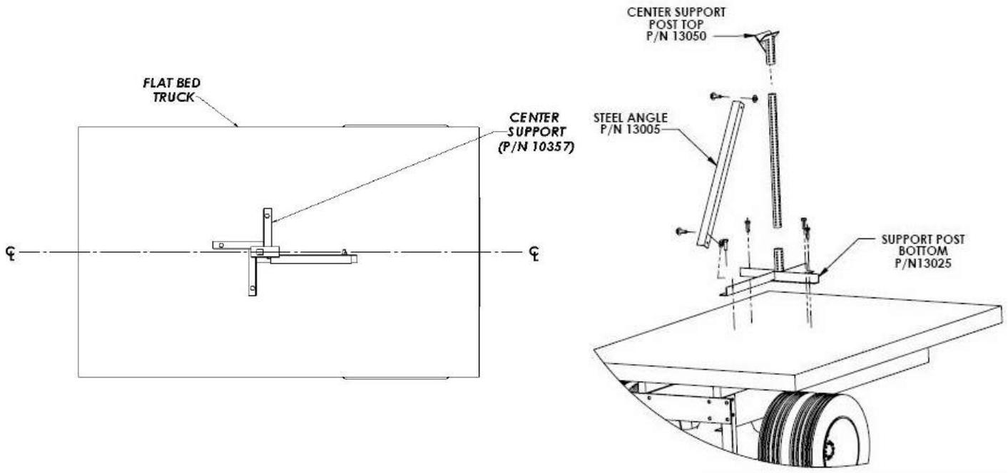
2. Make sure the angle located on the rear cartridge diaphragm aligns with the center support top post angle when the TMA is in the stored position, as shown in this bottom figure.
