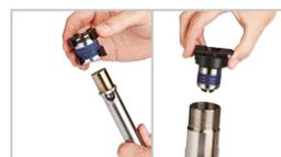
Insert pre-oiled packing cartridge assembly
