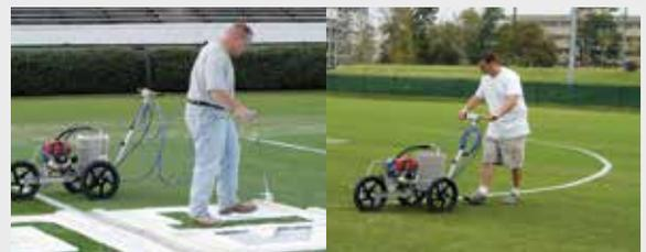
**No-Tool Gun Removal** for spraying stencils or large solid areas.
