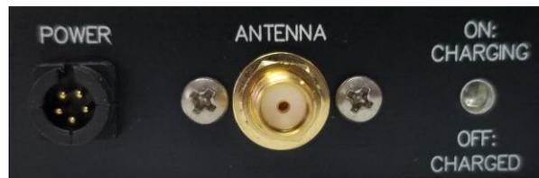
The internal batteries are charged by inserting the correct charger plug in to the end panel 'POWER' socket. During this time, the charge LED will turn ON. The LED turns OFF when batteries are fully charged.
