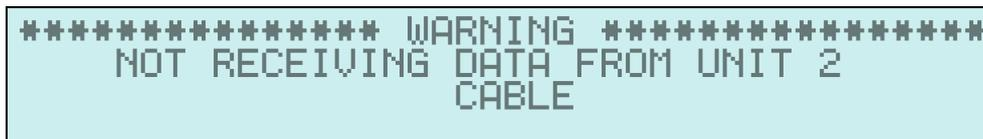
If the cable remains unplugged for more than 5 seconds, U1's screen will show the error:
